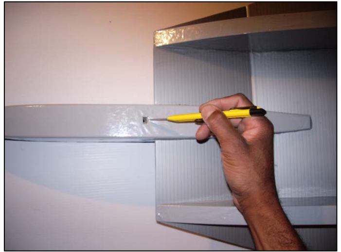
Cut slot for electronic speed control wires, it may be necessary to extend you electronic speed control battery wires in order to reach battery connector exit. Single knife cut is sufficient here, then use flat tip screw driver to open slot.
