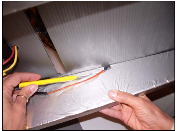
Cut slot in right nacelle for servo wire and extension, single knife cut is sufficient here.
