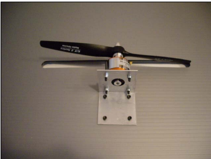
Bolt motor in place on wing using 4. 3mmX 14mm bolts, nuts and washers included. Prop slot can be trimmed if necessary. (TOP VIEW)
