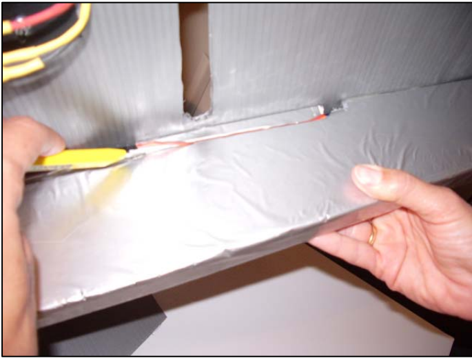
Embed servo wire and extension. Repeat steps for left side.
